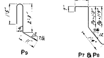
BENT BAR DETAILS Dimensions shown are out to out
