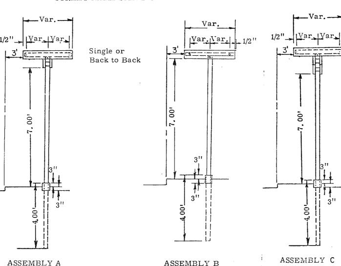
NOTE: The ground mounted street name sign areas have been calculated using a 6"x36" sign panel. The city shall determine the size needed and inform the Contractor of the exact length required to accommodate the message in accordance with the following legend.
